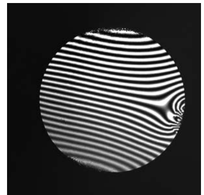
VFI 400µm calibration fiber viewed in fringe mode
