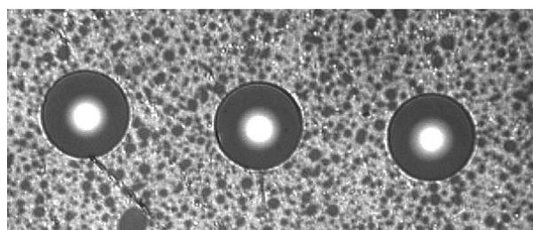
Interferogram of a ribbon cleave (image on the left) and inspect view of fibers in a multi-way ferrule (image on the right).
