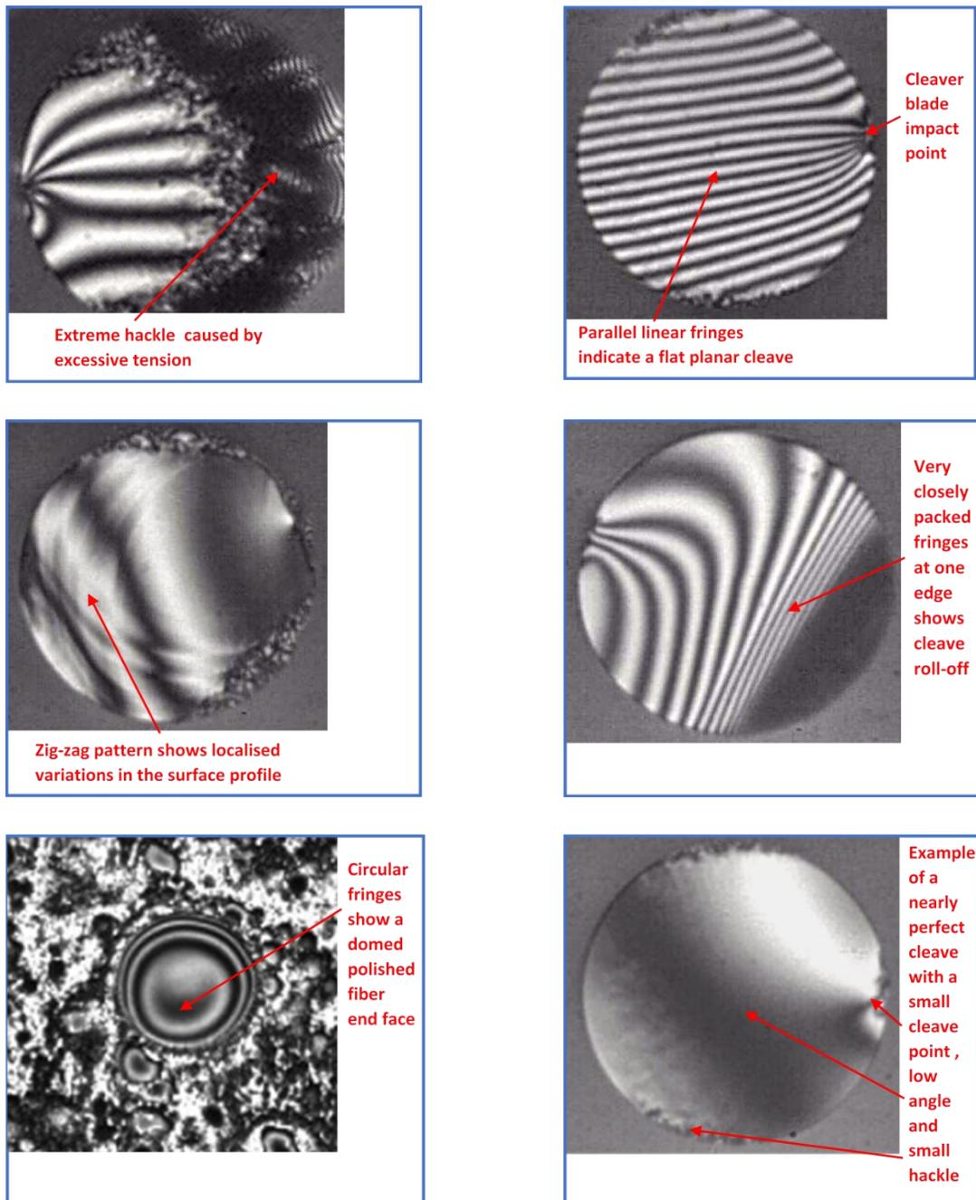
Figure 6 shows a typical 125 $\mu$ m fiber cleaved using the type of cleaver used in factories throughout the world. These 2 images taken together can yield a lot of information for the operator.
