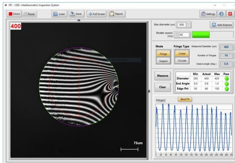
Figure 5 – 400 µm diameter fiber with end angle of 0.8 °
