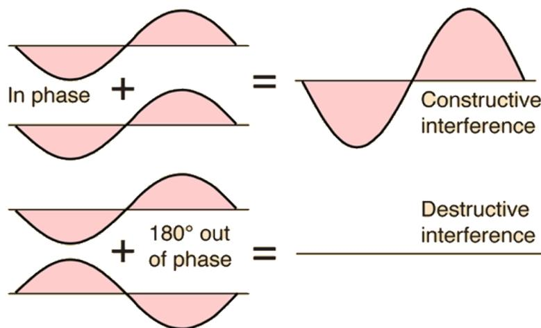
**Figure 2 – constructive and destructive interference**
